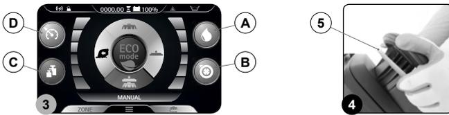
**NB:** if the button (3) is pressed when working in MANUAL MODE, the machine will shift to ECO-MODE, leaving the program in use at the time active (Fig. 2).
