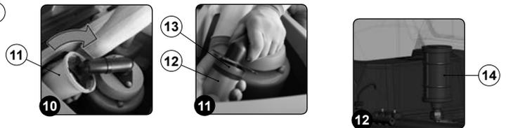
15. Rinse the recycle filter (14) thoroughly under the jet of the tank cleaning accessory.
