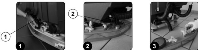
6. Remove the rear rubber-pressing blade by releasing the retainer (3) on the back of the squeegee (Fig. 4).
