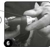
**NB:** to adjust the intensity of the solution jet from the tank cleaning accessory, turn the knob (7) on the accessory itself (Fig. 7).
