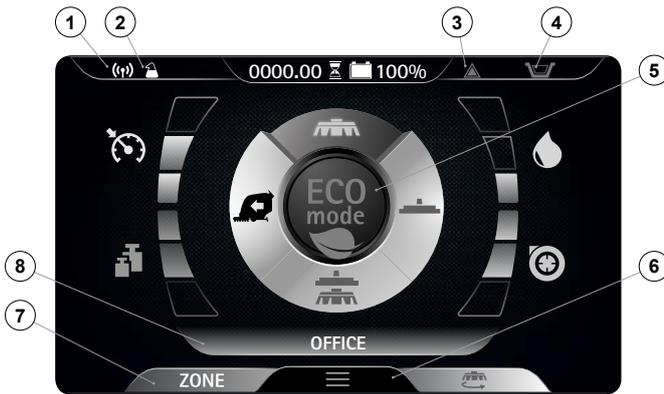
Selecting the program "SCRUBBING WITHOUT DRYING", the control display screen will appear as shown in the figure.
