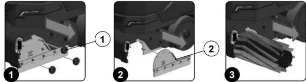
Careful cleaning of the brush guarantees better cleaning of the floor, as well as a longer brush head gearmotor lifespan. To clean the brush (with the optional spray gun kit), proceed as follows:
