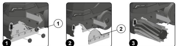
7. Replace the worn brush with the new one. Insert the brush into the tunnel (Fig. 4), taking care to make sure that the gearmotor's drive shaft enters the slit in the brush itself.
