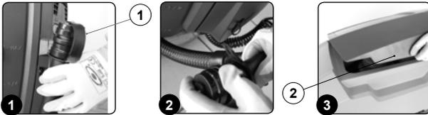
6. Release the tank cleaning accessory (3) (at the back of the machine) from the retainers (Fig. 4).
