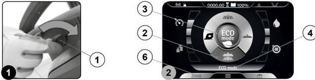
**NB:** by selecting one of the three working programs on the DS selector, ECO-MODE will be automatically activated.
