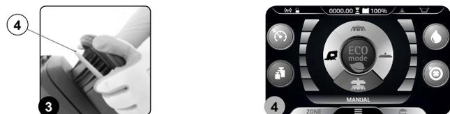
**(i) N.B.:** if the "ZONE" button (4) is pressed when working in ECO-MODE, the machine will shift to PROGRAM ZONE mode (Fig. 2); as soon as button (4) is pressed, the screen enabling you to select the working zone will appear on the display (Fig. 5).
