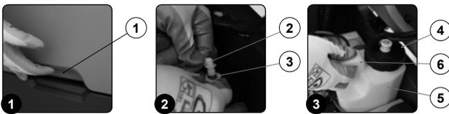
6. Remove the cap (4) from the detergent canister (Fig. 4).
