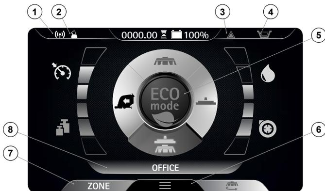
Selecting the program "SCRUBBING WITH DRYING", the control display screen will appear as shown in the figure.
