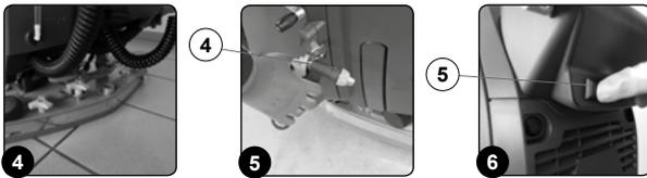
**NB:** before activating the optional tank cleaning kit, check the level indicator (6) to see how much solution there is in the recovery tank (Fig. 7).
