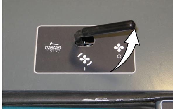
7. Push the hopper door lever forward to empty the hopper.
