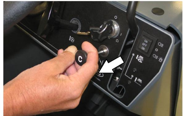
5. Turn the ignition switch key clockwise until the engine starts.
