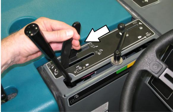
11. Move the vacuum and filter shaker lever into the **Vacuum fan on** position.
