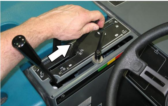
4. Move the vacuum and filter shaker lever to the **Vacuum fan on** position.
