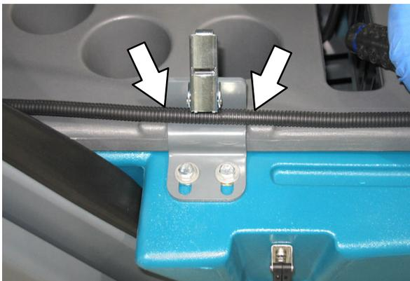
23. Reinstall the upper cyclone assembly, dust filter, and HEPA filter assembly in reverse order of disassembly.
