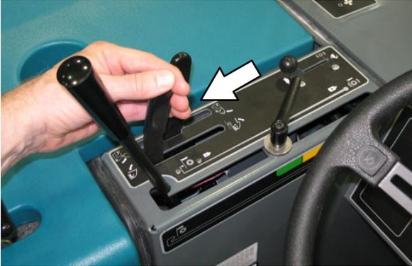
11. Push the hopper door lever forward to open the hopper door.
