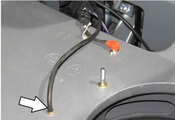
2. Disconnect the main wire harness from the filter shaker assembly and remove the filter shaker assembly from the filter compartment.
