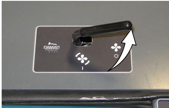
*NOTE: Excessive heat in the hopper will cause the Thermo Sentry to move the vacuum and filter shaker lever to the **Vacuum fan off** position. It will also make the hopper temperature light come on. If this happens, stop the machine, eliminate the source of the heat, and return the lever to the **Vacuum fan on** position.*
