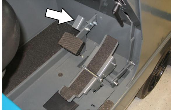
**NOTE:** If the operator is not in the seat, the parking brake must be engaged or the machine will automatically shut off after 2 seconds.
