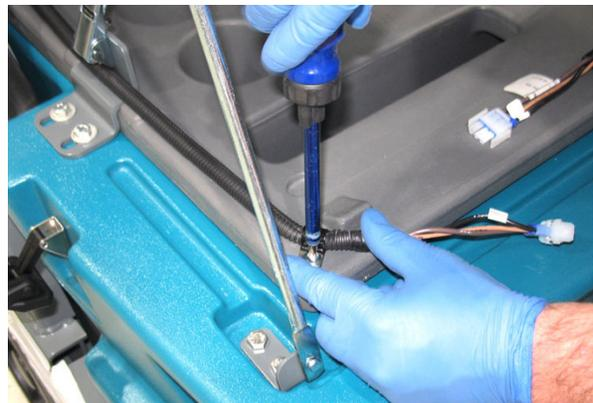
9. Remove the four brackets securing the lower cyclone chamber to the hopper.
