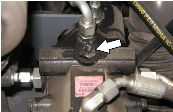
**ATTENTION! Do not push or tow machine for a long distance and without using the bypass valve, or the machine hydraulic system may be damaged.**
