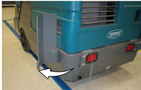
3. Close and secure the tower bumpers before operating the machine.
