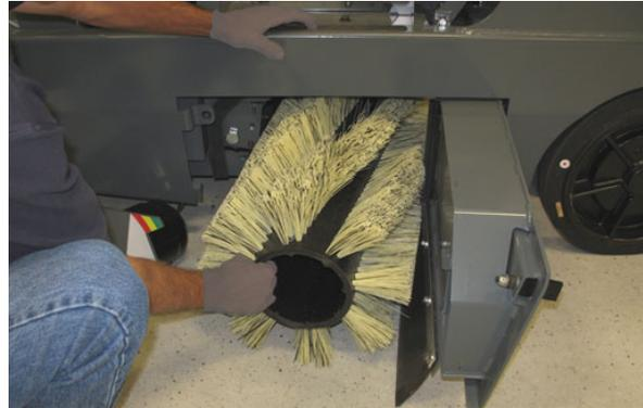
5. Replace or rotate the main brush end-for-end.
