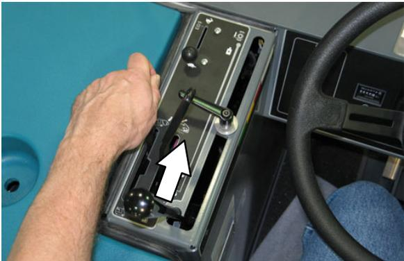
12. Move the vacuum and filter shaker lever into the **Vacuum fan on** position.
