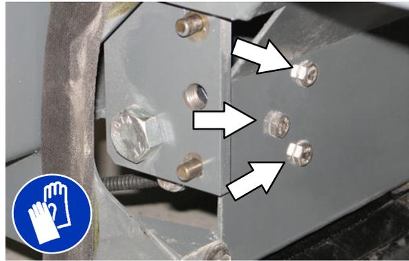
3. Move the bracket up or down in the slots and tighten the mounting bolts.
