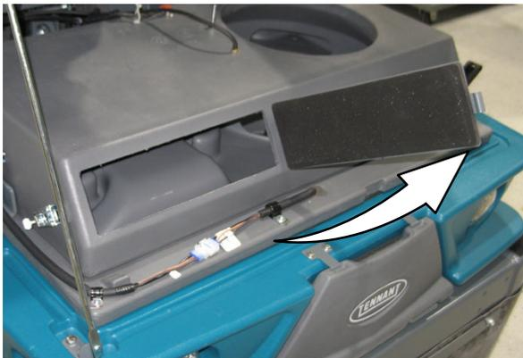
3. HEPA Machines: Use a HEPA certified vacuum to clean dust and debris from the interior of the upper cyclone chamber.
