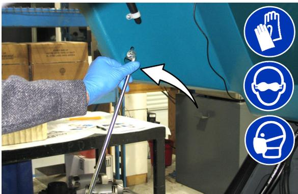
3. Completely loosen the two wing nuts securing the dust filter cover to the upper cyclone chamber.
