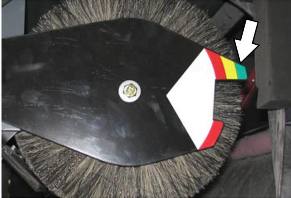
2. Loosen the main brush adjustment knob and slide the knob so it matches the color band on the brush idler plate. Retighten the knob.
