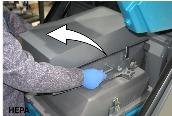
6. HEPA Machines: Clean and inspect the HEPA filter assembly seal for wear and damage. Replace the seal if it is worn or damaged.
