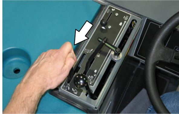
**FOR SAFETY:** When using machine, make sure adequate clearance is available before raising hopper.
