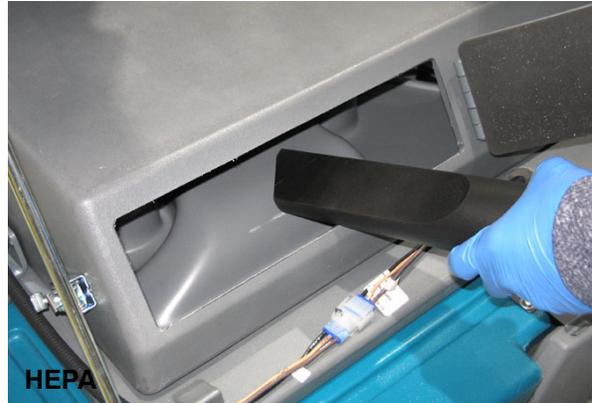
4. HEPA Machines: Use a HEPA certified vacuum to clean the slots located at the top of the dust filter compartment.
