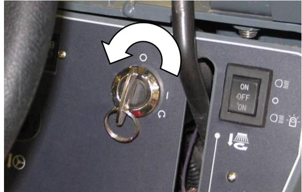
**FOR SAFETY: Before leaving or servicing machine, do not park near combustible materials, dust, gases, or liquids. Stop on level surface, set parking brake, turn off machine, and remove key.**
