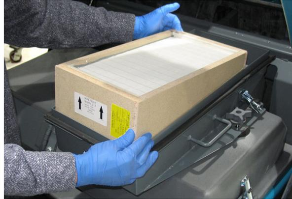
4. Inspect the HEPA filter and seals for dust, debris, and damage. Replace the HEPA filter if filter or filter seals are damaged.
