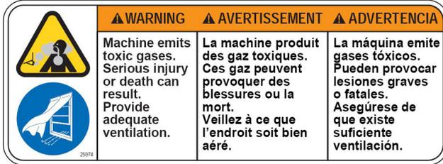
Located on the side of the operator compartment.
