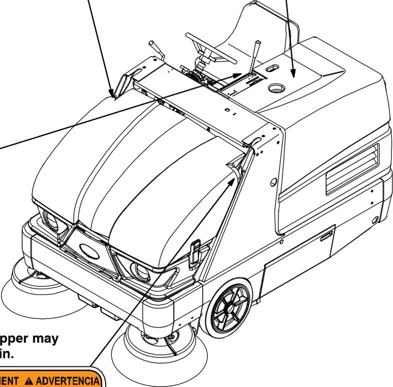
**WARNING LABEL – Raised hopper may fall. Engage hopper support pin.**
