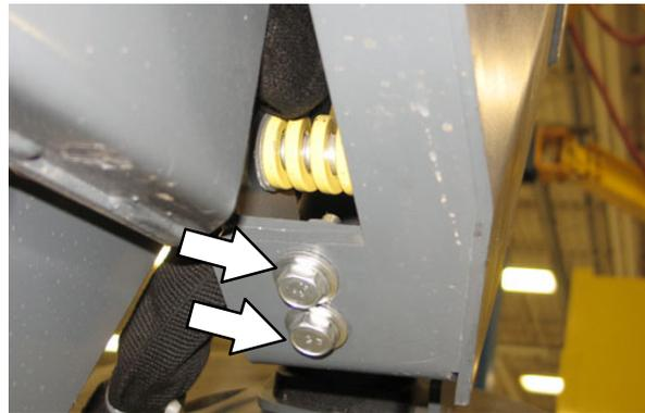
The side brush front to rear tilt is adjusted with the side brush cable and clevis pin.
