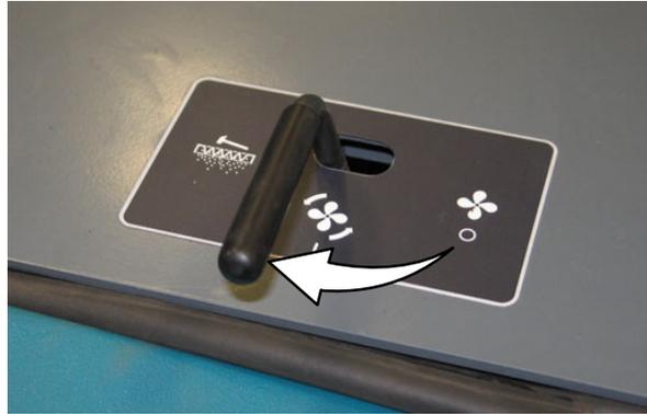
*NOTE: The vacuum fan duct should be off when sweeping wet debris.*
