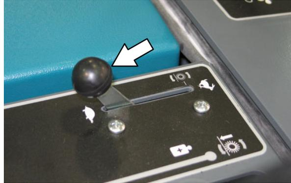
4. On gasoline powered machines, pull out the choke knob when the engine is cold. Push in the choke knob after the engine is running smoothly.
