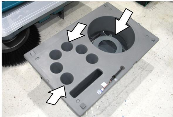
15. Inspect cyclone Perma-Filter inside the lower cyclone compartment for debris.
