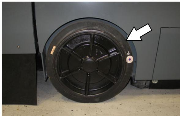
Check the front tires after every 100 hours of operation for damage. Check the rear tire pressure after every 100 hours of operation. The proper tire pressure is 795 kPa (115 psi).
