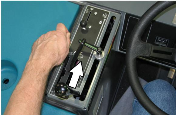
6. Move the throttle lever back into the **Idle engine speed** position.
