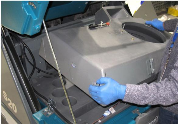
5. Inspect and clean the upper cyclone chamber seal. Replace seals if they are damaged or worn.
