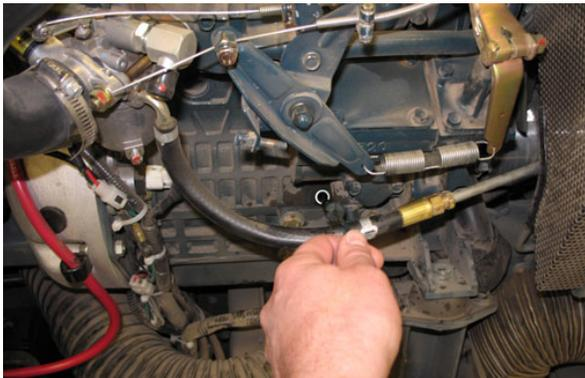
Fill the engine with oil until the oil is between the indicator marks on the dipstick. **DO NOT** fill past the top indicator mark. The engine oil capacity is 3.4 L (3.6 qt) with oil filter.
