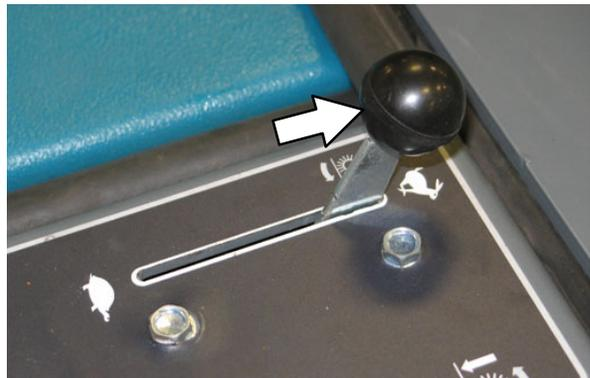
10. Pull and hold the hopper door lever back until the hopper door closed light comes on.
