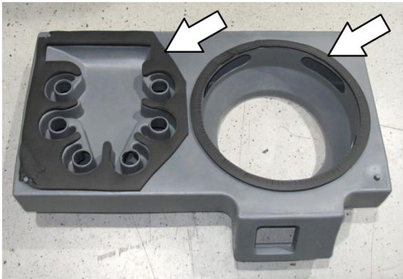
6. Inspect and clean the filter chamber inlet seal. Replace seal if they are damaged or worn.
