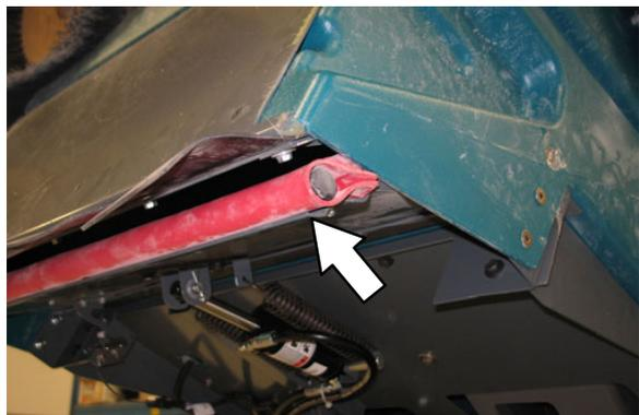
**FILTER CHAMBER INLET SEAL**
