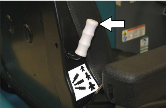
The backrest adjustment knob adjusts the angle of the backrest.
