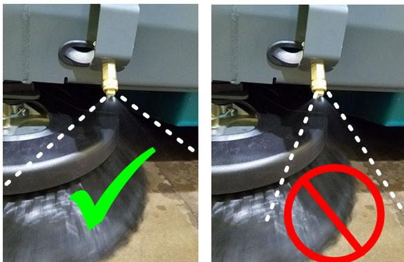
To adjust the spray pattern, use the water valve located next to the the water tank. Do not open the valve to the 90° maximum position. Optimal position is with the valve opened between 10–15°
