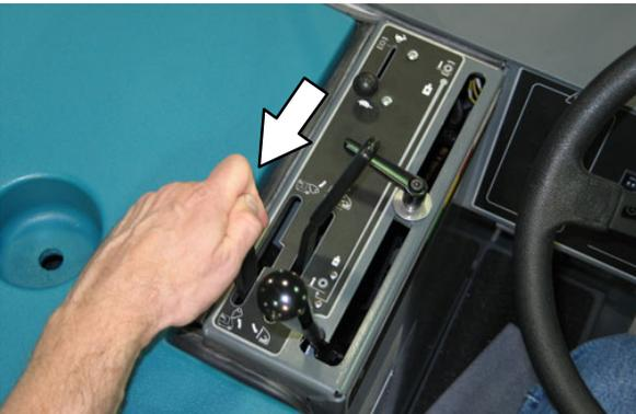
**FOR SAFETY: When using machine, do not raise hopper when machine is on an incline. Make sure adequate clearance is available before raising hopper.**
