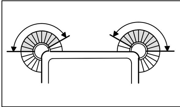
Turn the knob(s) counterclockwise to increase the brush pressure and clockwise to decrease the brush pressure.
