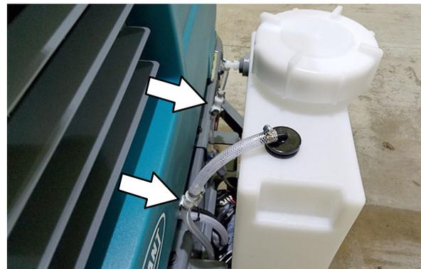
Disconnect the wire harness below the tank.
