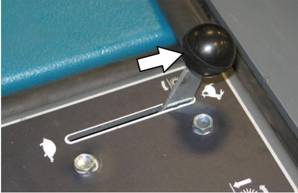
3. Push the hopper door lever forward to open the hopper door.
