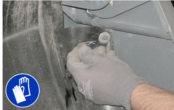
**WARNING:** Raised hopper may fall. Engage hopper support bar.
