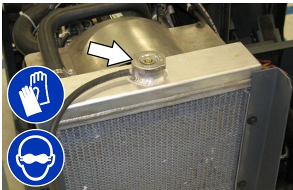
Check the radiator hoses and clamps after every 200 hours of operation. Tighten loose clamps. Replace damaged hoses and clamps.
