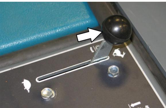
4. Pull and hold the hopper raise / lower lever back and raise the hopper to the desired height. Release the lever into the **Hold** position.
