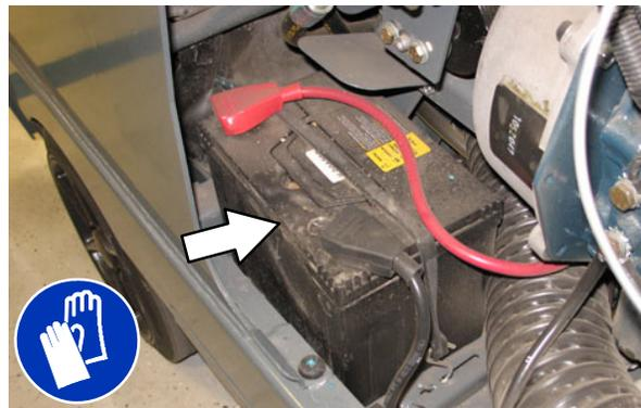
**FOR SAFETY:** When servicing machine, avoid contact with battery acid.
