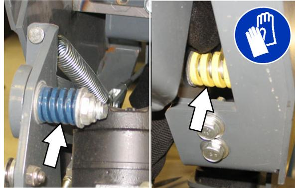
The side brush side tilt (left to right) is adjusted with the two bolts.
