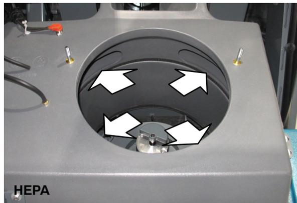
5. Close and secure the upper cyclone chamber access door when finished cleaning the interior of the upper cyclone chamber.
