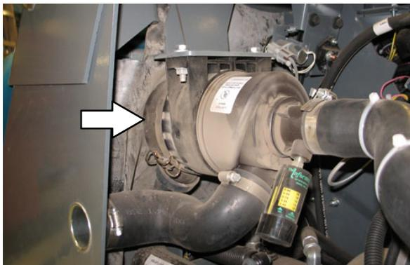
To remove the filter element, raise the hopper and engage the hopper support bar. Set the parking brake and turn the engine off. Remove the top two dust skirt clips and pull back the dust skirt to access the air filter housing.
