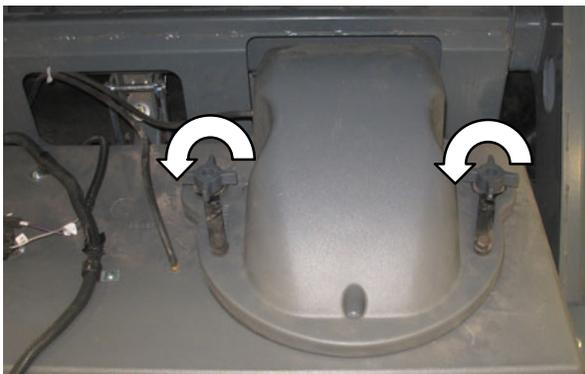
5. HEPA Machines: Remove the HEPA filter assembly.
