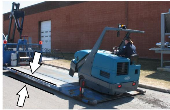
3. To winch the machine onto the truck or trailer, attach the winching chains to the rear tie down locations. The rear tie-down locations are the holes in the sides of the machine frame near the rear bumper.
