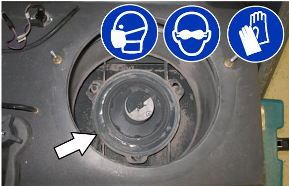
2. Machines (S/N 006266- ), open the front clean out door on the upper cyclone chamber and clean.
