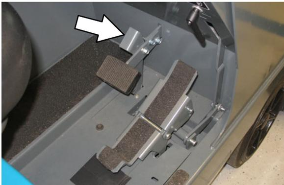
3. Move the throttle lever back into the **Idle engine speed** position.
