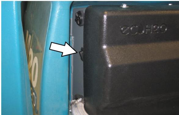
7. Press the *ec-H2O* module flush switch to shut off the system.
