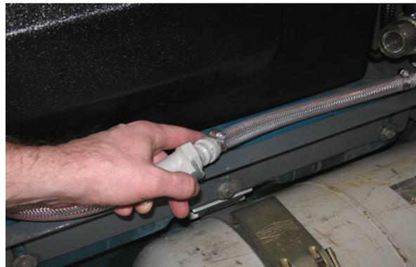
4. Pull the drain tube from the between the ec-H<sub>2</sub>O unit and the operator compartment, remove the cap from the tube, and place the end of the tube into an empty container. Set the cap aside.
