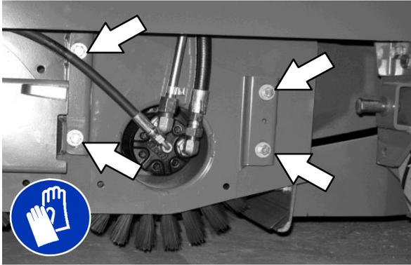
2. Move the brush drive housing up to decrease the pattern width on that side of the scrub head or down to increase the pattern width on that side of the scrub head.
