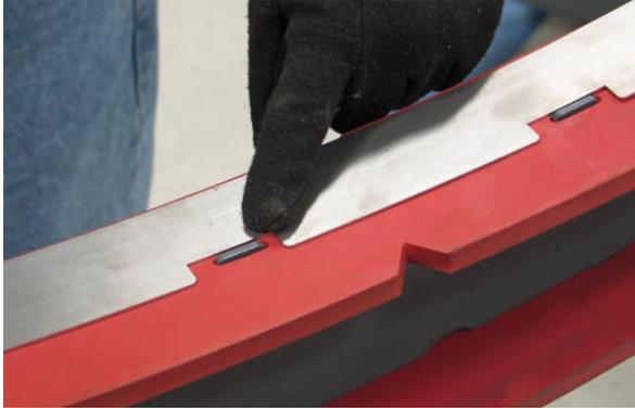
15. Tighten the front retaining band tension latch.
