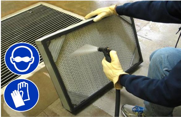
**NOTE:** If water is used to clean the dust filter, be sure the filter is completely dry before reinstalling it into the hopper. **Do Not** reinstall a wet dust filter.
