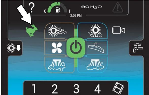
The *engine speed button* is off when the engine is in the low speed setting.
