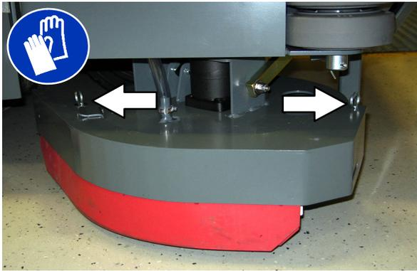
3. Open the retaining band tension latch.
