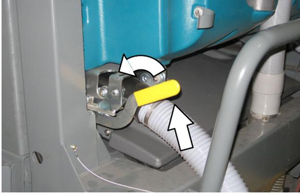
9. Reinstall the recovery tank drain hose onto the back of the recovery tank.
