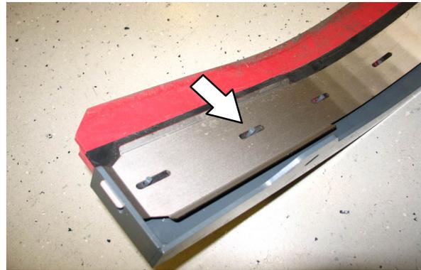
6. Reinstall the retaining band tension latch.
