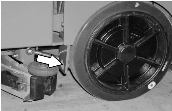
6. Route the tie-downs to the opposite ends of the machine and hook them to the brackets on the floor of the trailer or truck. Tighten the tie-down straps.
