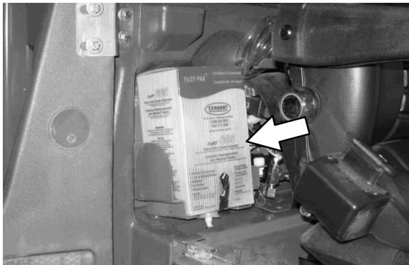
4. Remove the perforated knock outs from the new FaST-PAK carton. Do Not remove the bag from the carton. Pull out the hose connector located on the bottom of the bag and remove the hose cap from the connector.
