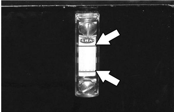
**ATTENTION! Do not overfill the hydraulic fluid reservoir or operate the machine with a low level of hydraulic fluid in the reservoir. Damage to the machine hydraulic system may result.**
