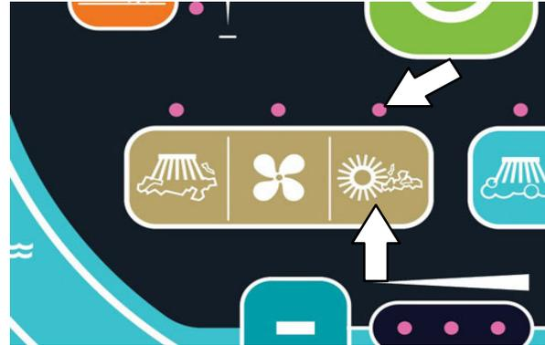
*NOTE: The sweeping mode and the scrubbing mode cannot both function at the same time. The sweeping mode will cease operating and the scrubbing mode will begin operating if any scrub button is pressed while the machine is in the sweeping mode.*
