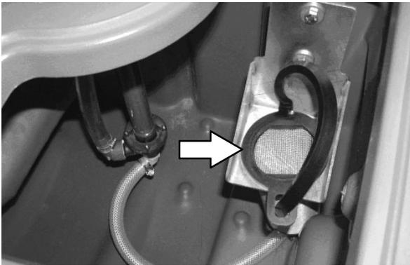
8. Rinse dirt and debris towards the recovery tank drain. Allow the recovery tank to drain.
