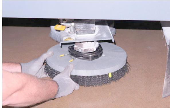
5. Set the brush spring open on the new brush to make installation easier.
