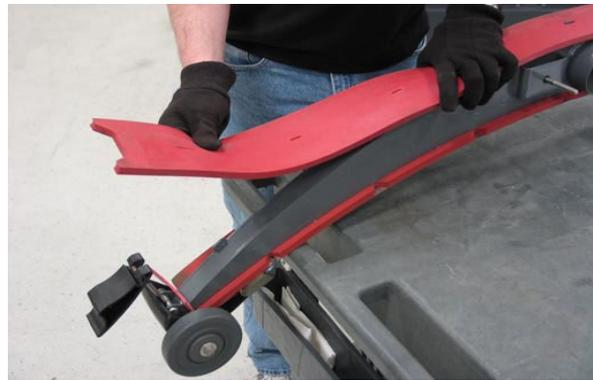
8. Install the new rear squeegee blade or rotate the existing blade to the new edge. Be sure all the holes in the squeegee blade are hooked onto the tabs.
