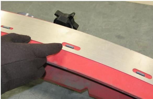
10. Tighten the rear retaining band tension latch.
