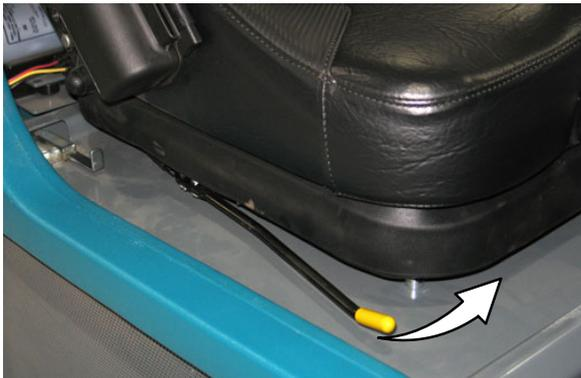
Adjust: Push to lever in towards the seat and slide the seat to the desired position. Release the lever to lock the seat into place.
