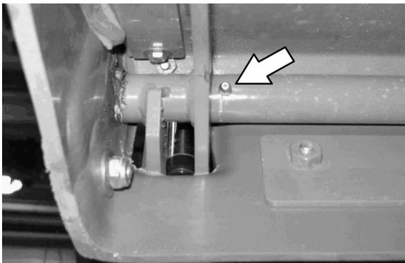
On the other side of the machine the torque tube grease fittings are located beneath the propel pump.
