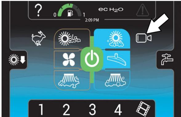
The camera automatically comes on when the bottom of the *directional pedal* is pressed to place the machine in reverse and remains on the entire time the machine is in reverse.
