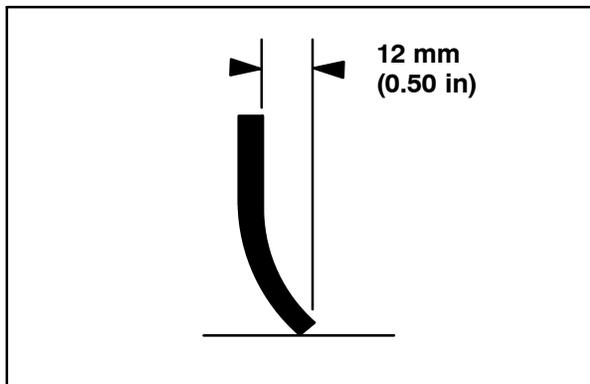
3. To adjust the overall squeegee blade deflection, turn the adjustment knobs counterclockwise to increase deflection or clockwise to decrease deflection.
