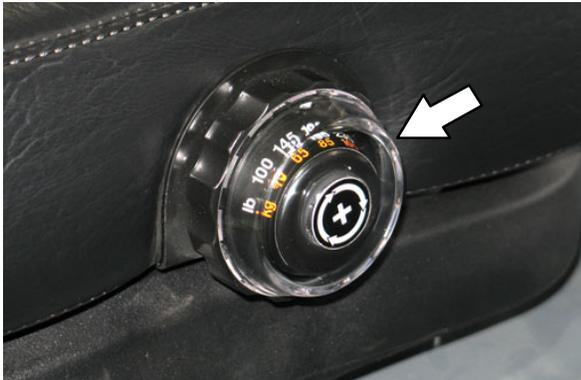
Increase firmness: Turn the weight adjustment knob clockwise.
