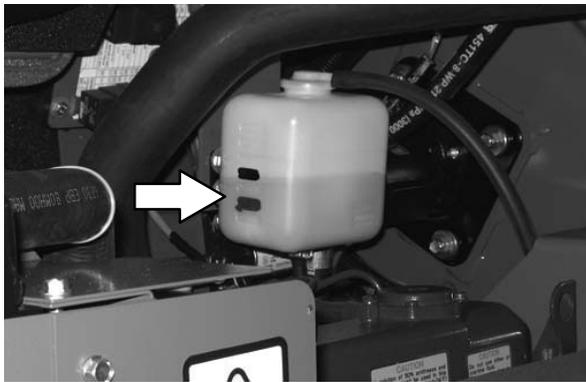
Flush the radiator and the cooling system after every 800 hours of operation.
