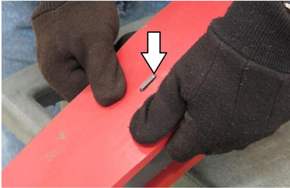
9. Reinstall the rear retaining band aligning the tabs with the holes.
