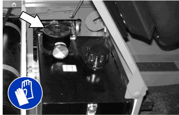
Replace the hydraulic strainer outlet after every 2400 hours of operation.
