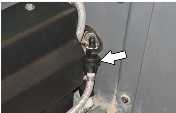
9. Blow pressurized air (less than 344 kPa (50 psi)) into the *ec-H2O* system outlet hose. Continue blowing compressed air into the outlet hose until water no longer drains from the drain tube
