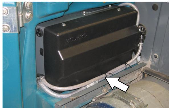
13. Return the intake flush hose to the storage bag behind the operator seat.
