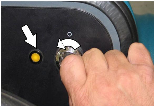
3. Turn the key clockwise to start the engine.
