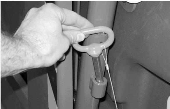
5. Insert the hopper support pin into one of the three hopper support holes. Lower the hopper until it rests on the support pin.
