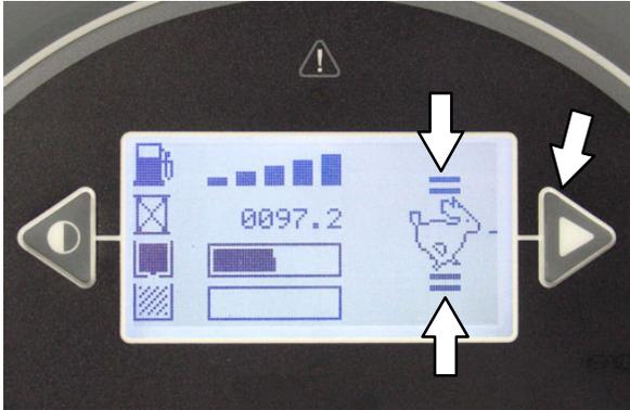
When two thicker bars appear above and below the engine speed icon and the thinner bars and the icon is solid the engine is in the high setting.
