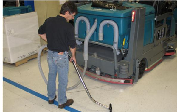
8. When finished vacuuming, press the *Scrub vacuum fan/squeegee* button to turn off the vacuum. The light above the button will turn off.
