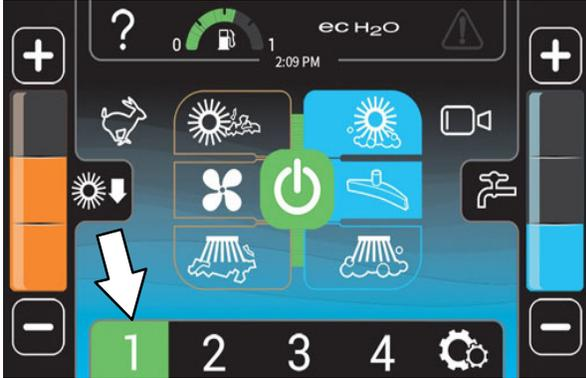
5. Press the yes button to set the zone settings. Press the no button to return to the main operating screen.
