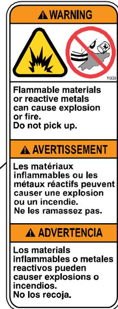
Located on the side of the operator compartment.
