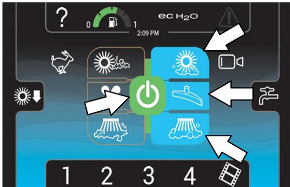
*NOTE: DO NOT turn on the FaST or ec-H2O system during conventional scrubbing. Conventional cleaning detergents could cause a FaST or ec-H2O system failure. Drain, rinse, and refill the solution tank with cool clean water before operating the FaST or ec-H2O system.*
