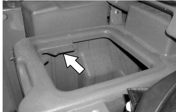
2. Open the recovery tank cover and fill the recovery tank with water (not to exceed 60°C / 140°F) until the recovery tank is approximately half full.
