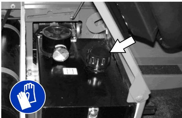
Replace the hydraulic fluid filter after every 1200 hours of operation or if the hydraulic reservoir gauge is in the yellow/red zone when the reservoir hydraulic fluid is approximately 32° C (90° F).
