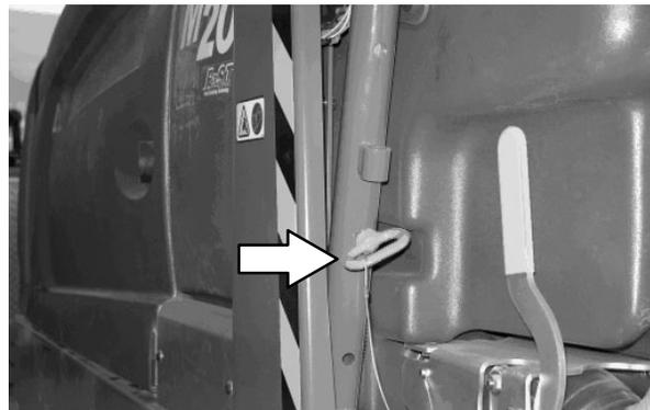
**WARNING:** Raised hopper may fall. Engage hopper support pin.
