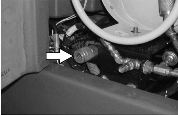
2. Turn the ignition switch to the on position (without starting) and turn on the water source. The auto-fill automatically fills the tanks to the proper level.
