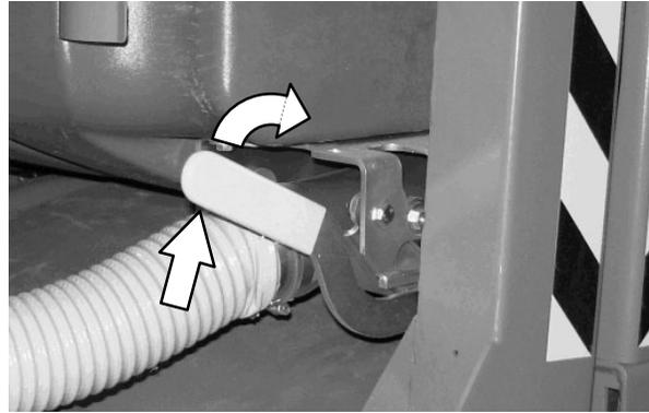
7. Reinstall the solution tank drain hose onto the back of the recovery tank.
