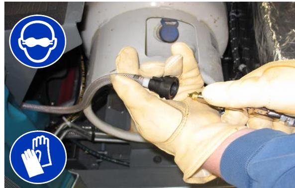
10. Reinstall the cap onto the drain tube and insert the tube back between the *ec-H2O* module and the operator compartment.
