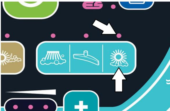
**NOTE: NOTE:** The scrubbing mode and the sweeping mode cannot both function at the same time. The scrubbing mode will cease operating and the sweeping mode will begin operating if any sweep button is pressed while the machine is in the scrubbing mode.
