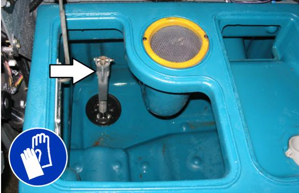
4. Open the recovery tank Variable Drain Valve.
