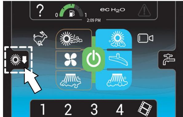
Use the brush pressure increase (+) button and the brush pressure decrease (-) button to change the brush pressure. The brush pressure indicator bar displays the current brush pressure setting.
