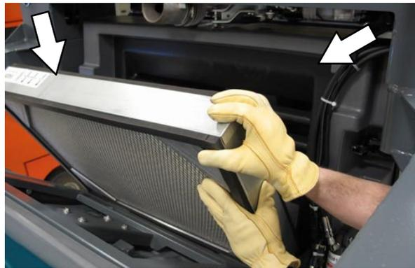
8. Clean or discard the dust filter. See the *CLEANING THE HOPPER DUST FILTER* section of this manual.
