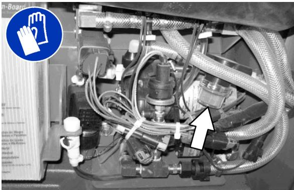
**REPLACING THE FaST SYSTEM FILTERS**
