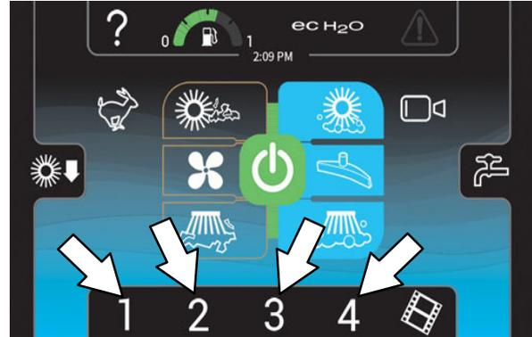
Press the required zone control button. The selected preset button will illuminate and the name of the zone appears above the button. The *solution flow indicator bar* / adjustment buttons and *brush pressure indicator bar* / adjustment buttons briefly appear in the display to show the settings for the selected zone.
