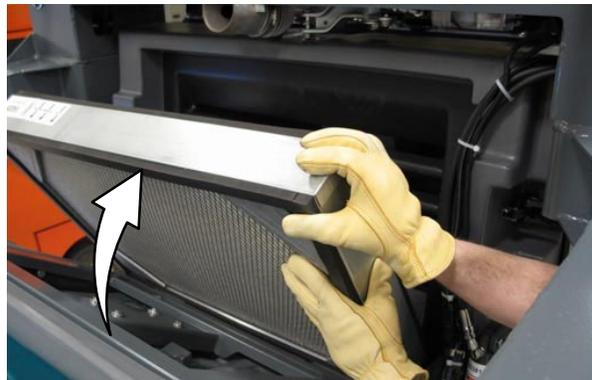
11. Close the filter cover and secure the filter cover to the hopper with the handles.
