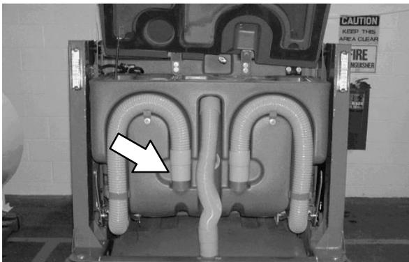
3. Open the recovery tank Variable Drain Valve.
