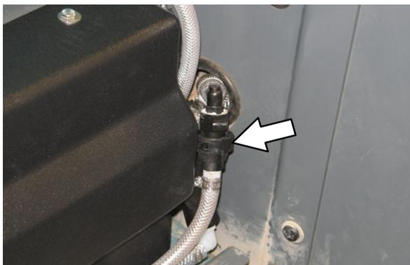
5. Place the *ec-H2O* system intake hose into a container containing 5 gallons (19 liters) of white or rice vinegar. Place the outlet hose into an empty bucket.
