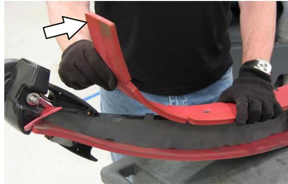
13. Install the new front squeegee blade or rotate the existing blade to the new edge. Be sure the holes in the squeegee blade are hooked onto the tabs.
