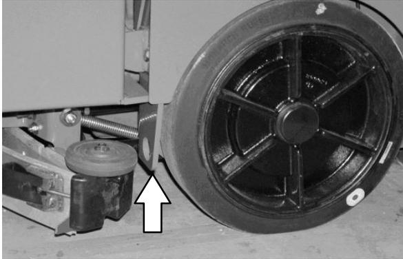
Front jacking locations are located on the frame directly in front of the front tire.
