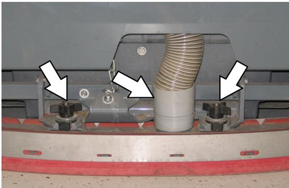
3. Remove both mounting knobs from the rear squeegee assembly.
