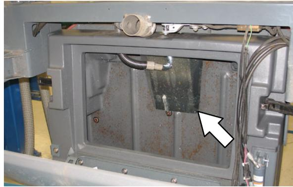
10. Reinstall the hopper dust filter. See **REMOVING THE HOPPER DUST FILTER** section of this manual.
