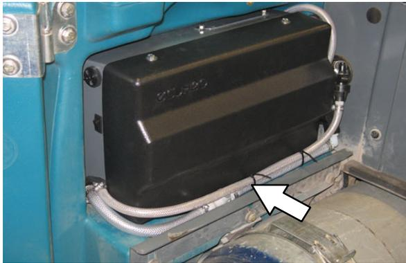
*NOTE: The outlet and intake hoses must be down between the *ec-H2O* assembly and the bracket so they are not pinched or damaged when the operator seat cover is closed.*
