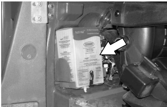
When in the optional ES (Extended Scrub) mode, the dirty solution in the recovery tank is filtered through the ES system and returned to the solution tank for reuse. Detergent is then injected into the returned solution to revitalize the cleaning capability of the solution.
