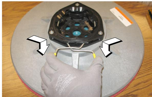
6. Place the new side brush underneath the side brush assembly and lift the side brush up onto the side brush hub until the brush locks onto the hub.
