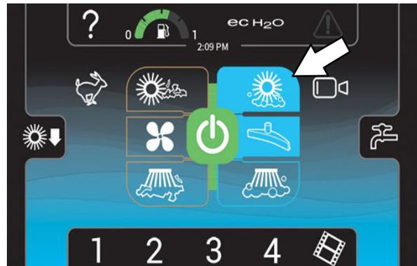
**NOTE:** The scrubbing mode and the sweeping mode cannot both function at the same time. The scrubbing mode will cease operating and the sweeping mode will begin operating if any sweep button is pressed while the machine is in the scrubbing mode.
