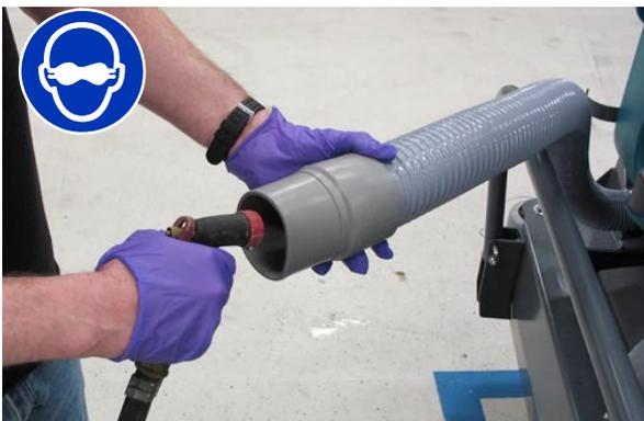
6. Rinse dirt and debris out the open drain.
