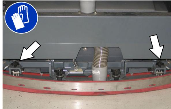
4. Drive the machine forward again to recheck the squeegee blade deflection after adjustments are made.
