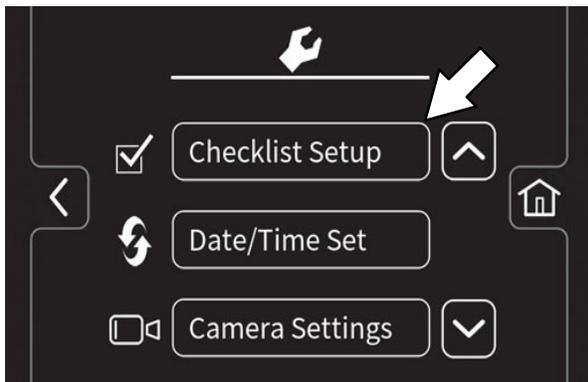
3. Press the Disable Checklist button / Enable Checklist button to disable / enable the Pre-Operation Checklist.
