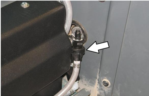
4. Place the *ec-H2O* system outlet hose into an empty container.
