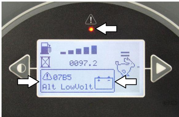
The LCD will display a fault / alert code. If there is more than one fault, each fault code will alternately display.
