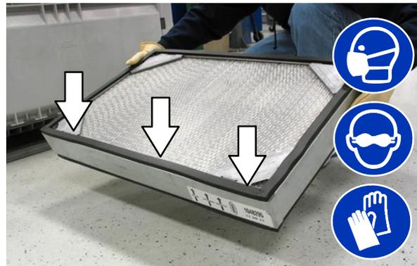
**AIR**—Always wear eye protection when using compressed air. Blow air through the dust filter opposite the direction of the arrows. Never use more than 690 kPa (100 psi) of air pressure and never hold the nozzle closer than 50 mm (2 in) to the filter. This may be done with the dust filter in the machine.
