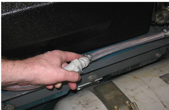
4. Disconnect the *ec-H2O* system outlet hose from the hose to the scrub head and connect the outlet flush hose (black connector) to the *ec-H2O* system outlet hose.
