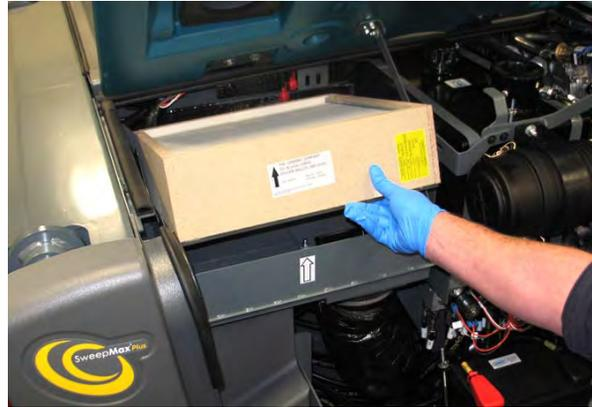
4. Inspect the HEPA filter and seals for dust, debris, and damage. Replace the HEPA filter if filter or filter seals are damaged.
