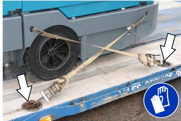
**FOR SAFETY: When unloading machine off truck or trailer, use winch. Do not drive the machine off the truck or trailer unless the loading surface is horizontal AND 380 mm (15 in) or less from the ground.**
