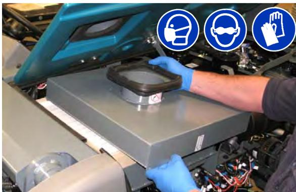
3. Remove the HEPA filter from the HEPA filter compartment.
