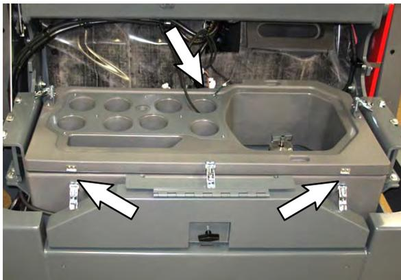
8. With the help of an assistant, lift the lower cyclone chamber and remove it from the hopper.
