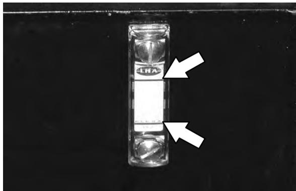
A filler cap is mounted on top of the reservoir. It has a built-in breather and fluid level dipstick. Replace the cap after every 800 hours of operation.
