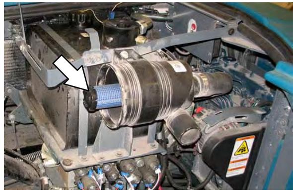
Install the filter element into the air filter housing and reinstall the dust cap with the water drain pointing down.
