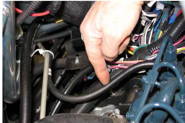
The rubber fuel lines can become worn-out whether the engine has been used much or not. Replace the fuel lines and clamp bands every two years.
