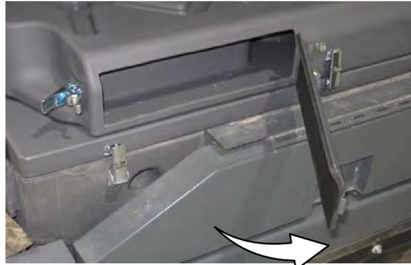
4. HEPA Machines: Use a HEPA certified vacuum to clean dust and debris from the interior of the upper cyclone chamber.
