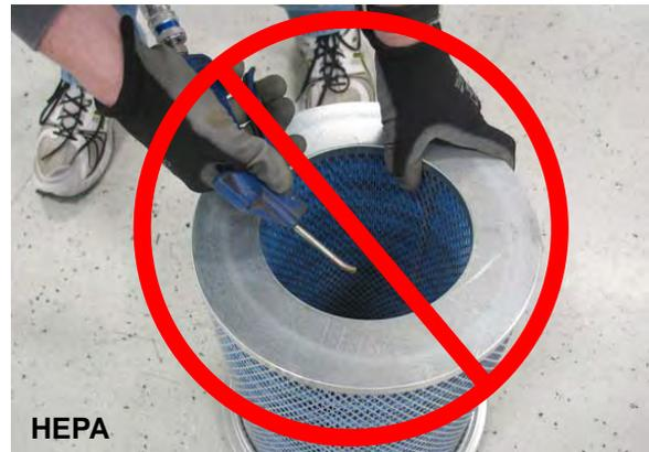
Inspect the dust filter seals for proper seal and damage. Dust build up on the seal surfaces means dust is getting past the dust filter, significantly reducing the HEPA filter life.
