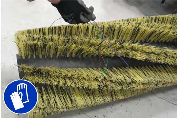
Rotate the brush end-for-end after every 50 hours of operation, for maximum brush life and best sweeping performance. Refer to *REPLACING OR ROTATING THE MAIN BRUSH*.
