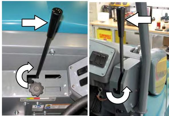
8. Release the *parking brake*, then press the *Directional pedal* to begin sweeping.
