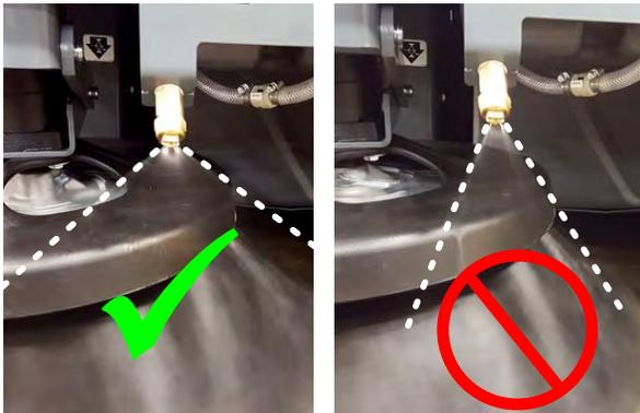
To adjust the spray pattern, use the water valve located under the water tank. Do not open the valve to the 90° maximum position. Optimal position is with the valve opened between 10–15°
