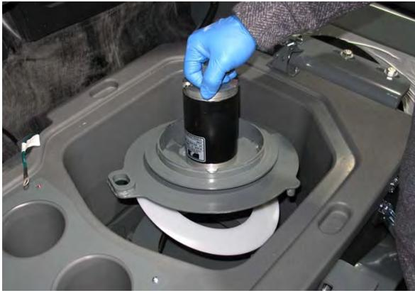
7. Loosen the three clamps securing the lower cyclone chamber to the hopper.
