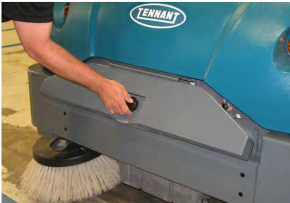
Pull the hopper access door handle to open the hopper access door. (SN 006501 – )
