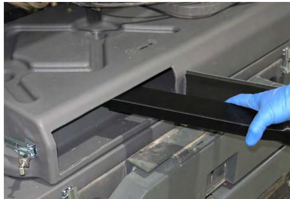
5. HEPA Machines: Use a HEPA certified vacuum to clean the slots located at the top of the dust filter compartment.
