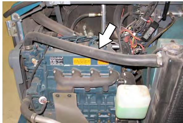
Check the radiator core exterior and hydraulic cooler fins for debris after every 100 hours of operation. Blow or rinse (with low pressure air or water) all dust through the grille and radiator fins, in the opposite direction of normal air flow. Be careful to not bend the cooling fins when cleaning. Clean thoroughly to prevent the fins from becoming encrusted with dust. To avoid cracking the radiator, allow the radiator and cooler fins to cool before cleaning.
