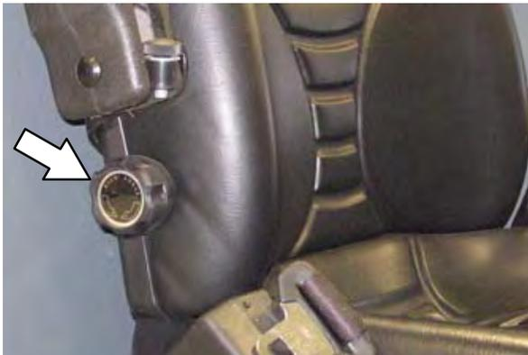
The front-to-back adjustment lever adjusts the seat position.
