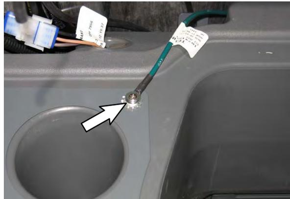
5. Disconnect the jumper harness from the filter shaker assembly.
