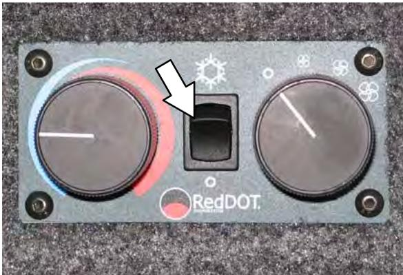
Use the *Temperature knob* to control the cab heater temperature. Use the *Fan knob* to control the air conditioner temperature.
