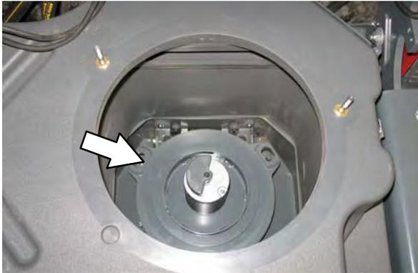
2. Open the rear cyclone cover access port to empty dust and debris from the cyclone cover.
