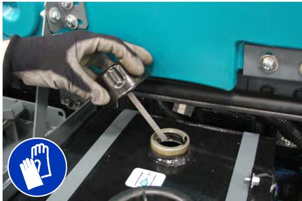
Machines (S/N 007685– ) have a fluid level gauge on the hydraulic tank. The hydraulic fluid level should be between the two lines on the hydraulic gauge.
