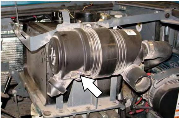
Remove the filter element. Carefully clean the end cap and the interior of the housing with a damp cloth. Clean the housing sealing surfaces.
