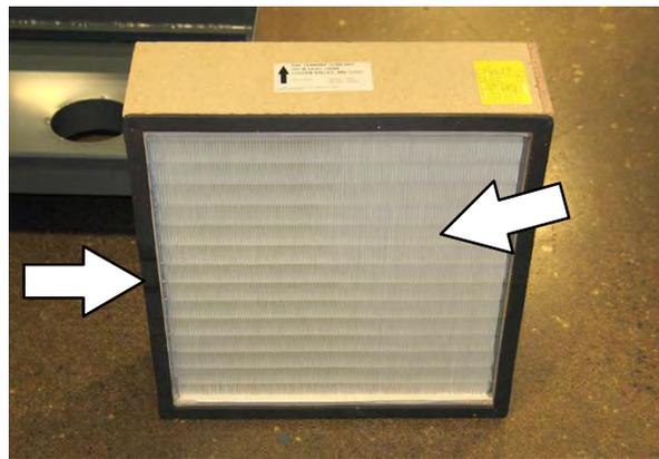
5. Use a HEPA certified vacuum to clean the HEPA filter compartment and the HEPA filter housing inlet hose.
