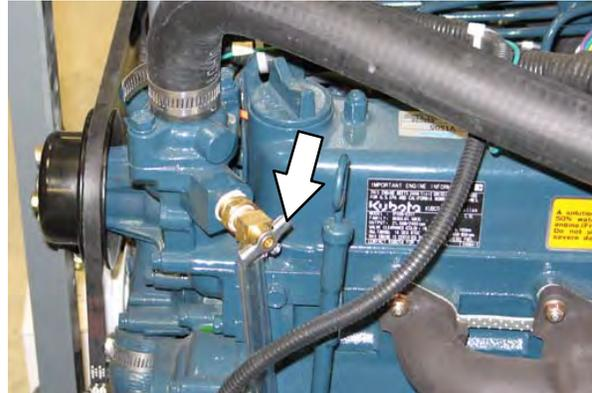
Check the radiator hoses and clamps after every 200 hours of operation. Tighten loose clamps. Replace damaged hoses and clamps.
