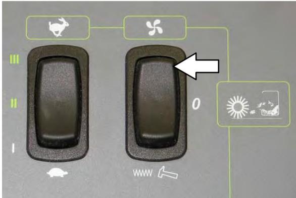
4. Ensure the *hopper door switch* is in the upper automatic position.
