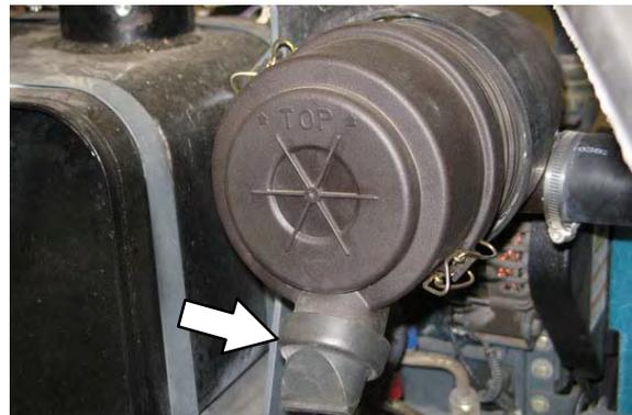
Push the reset button on the end of the indicator to reset the air filter indicator after replacing the air filter element.
