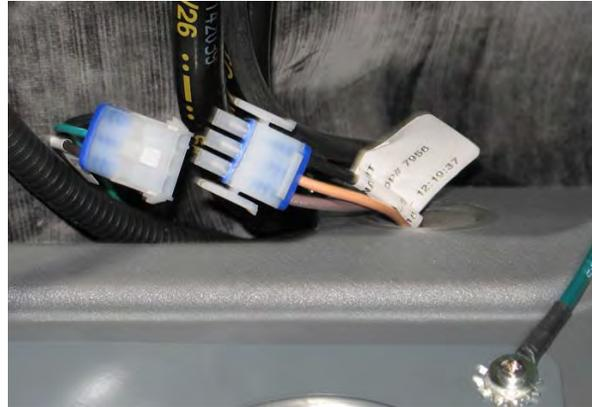
4. Disconnect the ground wire from the lower cyclone chamber.
