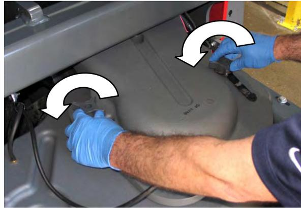
4. Disconnect the vacuum hose from the dust filter cover.
