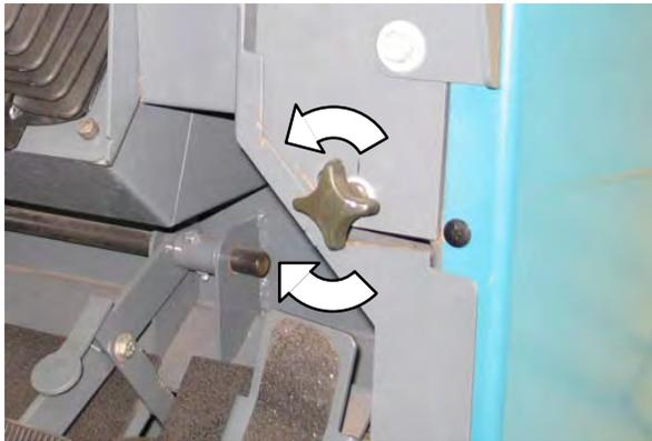
**S30 XP and X4:** Tighten the *side brush adjustment knob* into the side brush bracket to decrease brush pattern and loosen the knob to increase the brush pattern.
