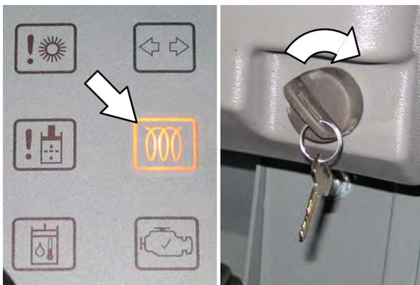
4. Turn the key further clockwise to start the engine.
