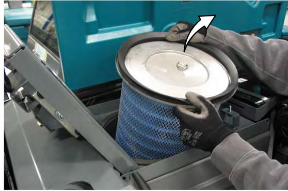
4. Clean or discard the dust filter element. Refer to *CLEANING THE DUST FILTER*.
