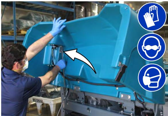
3. Completely loosen the two wing nuts securing the dust filter cover to the upper cyclone chamber.
