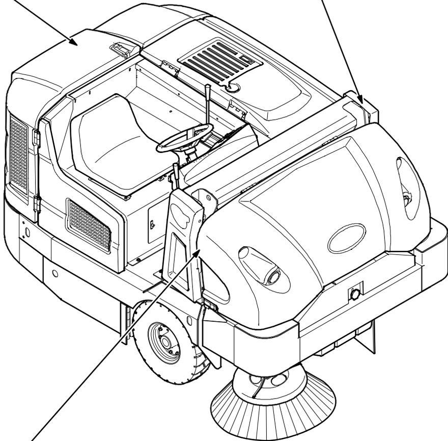
**WARNING LABEL – Raised hopper may fall. Engage hopper support bar.**
