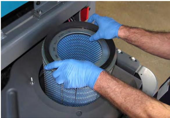
8. Clean or discard the dust filter element. Refer to *CLEANING THE DUST FILTER*.
