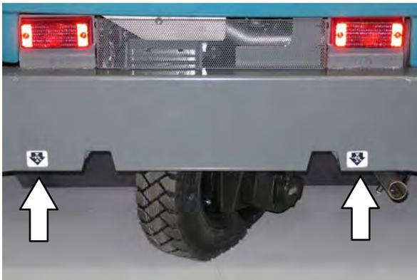
Front jacking locations are located on the frame directly in front of the front tire.
