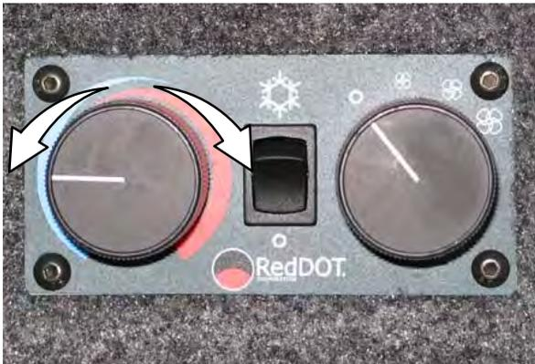
Use the *Fan knob* to control the fan speed. This knob affects the heater and air conditioner.
