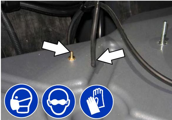
2. Loosen clamps securing the upper cyclone chamber and then remove it from the hopper.
