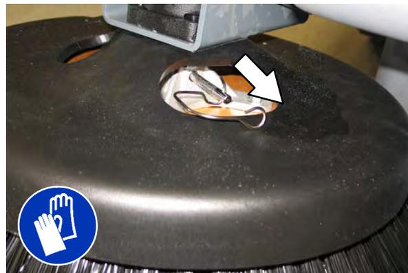
*NOTE: Remove the drive hub and put it on the new brush if one is not installed.*
