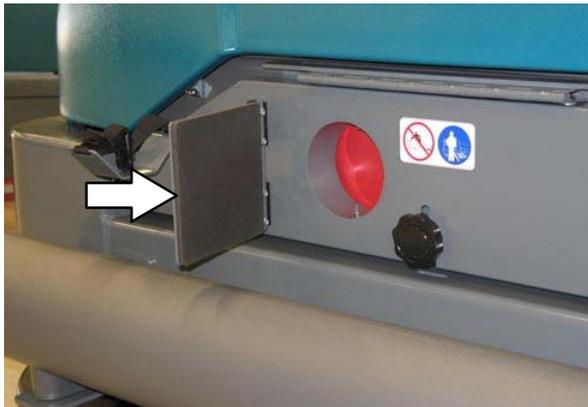
5. Attach the *blower wand* hose to the machine under the blower wand door located on the left side of the machine. Make sure the hopper door is open when operating the blower wand.
