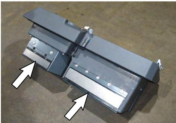
17. Allow the lower cyclone compartment / dust filter compartment / Perma-Filter compartment to completely dry.
