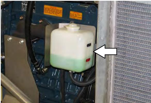
**FOR SAFETY:** When servicing machine, do not remove cap from radiator when engine is hot. Allow engine to cool.
