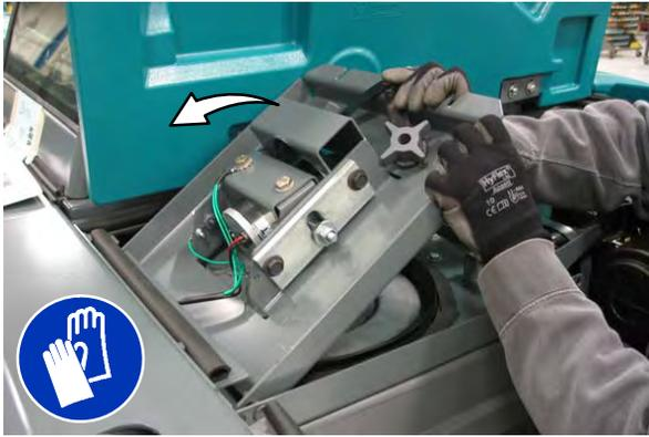
3. Remove the dust filter from the filter housing.
