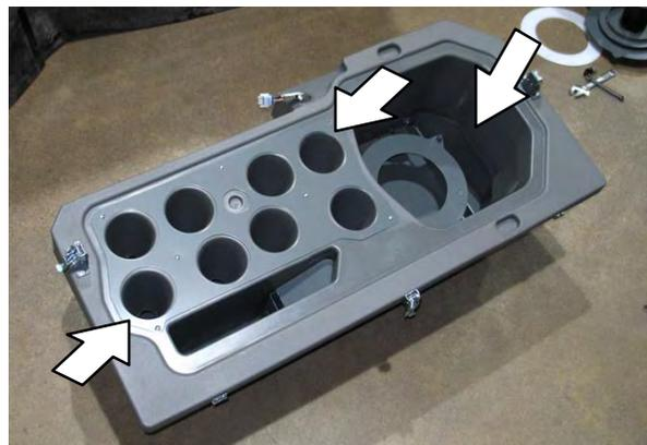
13. Inspect cyclone Perma-Filter inside the lower cyclone compartment for debris.
