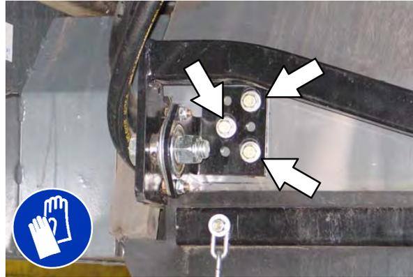
2. Move the bracket up or down in the slots and tighten the mounting bolts.
