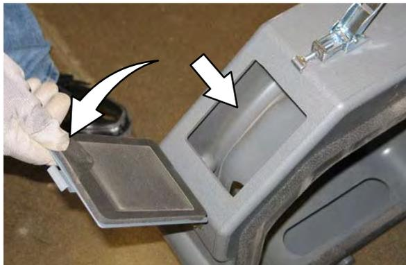
3. Machines (S/N 008826 - ), open the front clean out door on the upper cyclone chamber and clean.
