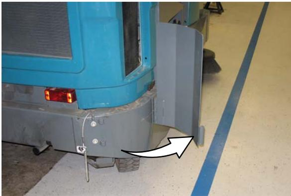
3. Close and secure the tower bumpers before operating the machine.
