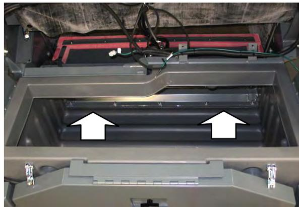
12. Use a garden hose to clean out the filter compartment and lower cyclone compartment.
